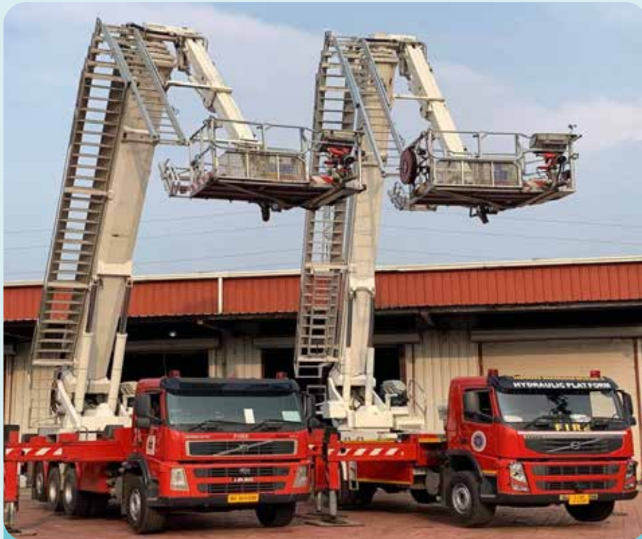
Incorporating advanced fire fighting vehicles such as 70 m ALP and 54m, 32m TTL in fire department
