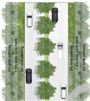
Figure 1 Typical Plan for 18-30m Wide Road
