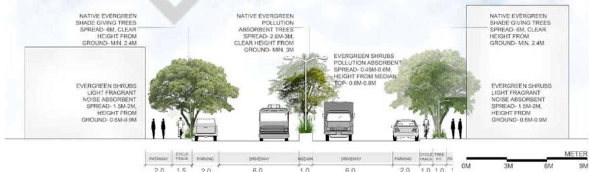
Figure 24: 3 Typical Sections for 18-30m wide road in PCMC
